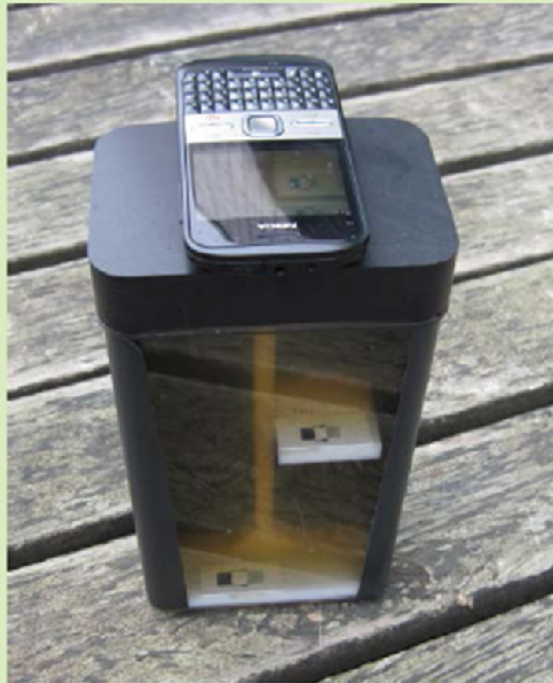
Fig. 1. Secchi3000 and a mobile phone on the top of the device. Inside the container there is the measurement structure with plates consisting of white, grey and black target areas.
